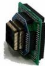
ICE Test Pod Courtesy of Signum Systems
